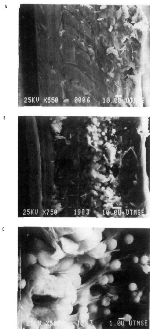
Figure 1. Scanning electron micrographs showing cross-sectional views of Nafion membrane: (A) Nafion ( \times 550 ), (B) Nafion loaded with CdS ( \times 750 ), (C) detail, as in (B), ( \times 5000 ). Calibrating bars are 10.0, 10.0, and 1.0 \mu\text{m} , respectively.
